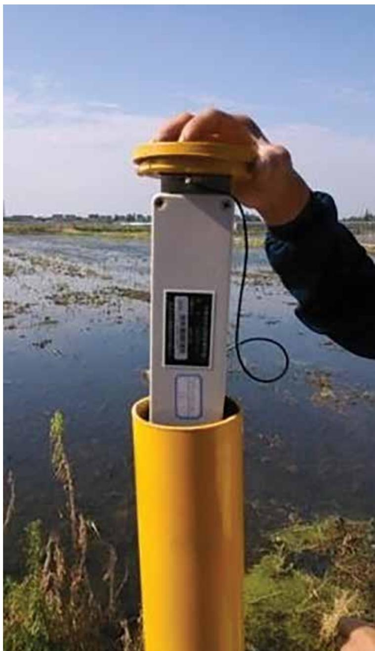
**Figure 9.** Intelligent data sampling units installed in test posts along the pipeline.
